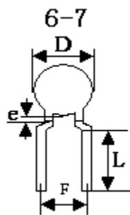
引线形式代码 Lead style code: 7 Unit: mm
