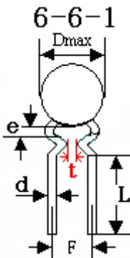
引线形式代码 Lead style code: 6 Unit: mm
