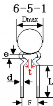
引线形式代码 Lead style code: 5 Unit: mm
