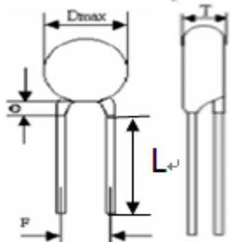
引线形式代码 Lead style code: 2 Unit: mm
