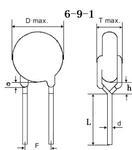
引线形式代码 Lead style code: 0 Unit: mm
